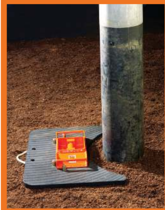
Place base plate onto the pole puller pad.
