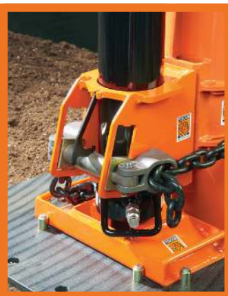
Lift the latch hook and allow the main load bar to drop which will pre-tension the chain.
