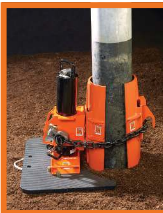
Confirm that the chain is in direct contact with the radius of the fixed back plate.
