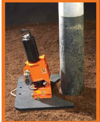
Place the swivel & hook assembly over the cylinder.
