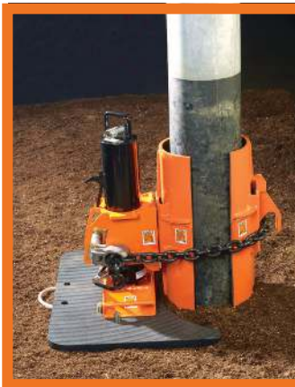
Take the 8 foot chain around the back side of the steel clamshell with fixed back plate.
