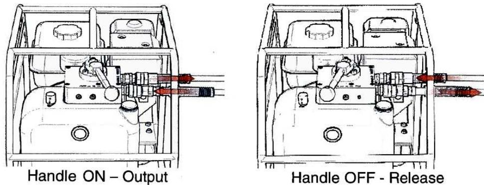
10. It is a good idea to check the pump output pressure before starting your task. Run the attached head while watching the pressure gauge near the pump handle. As the pump builds pressure the gauge will read the amount shown. The needle should reach 10,000 PSI before the bypass cartridge automatically releases and drops back to zero.
