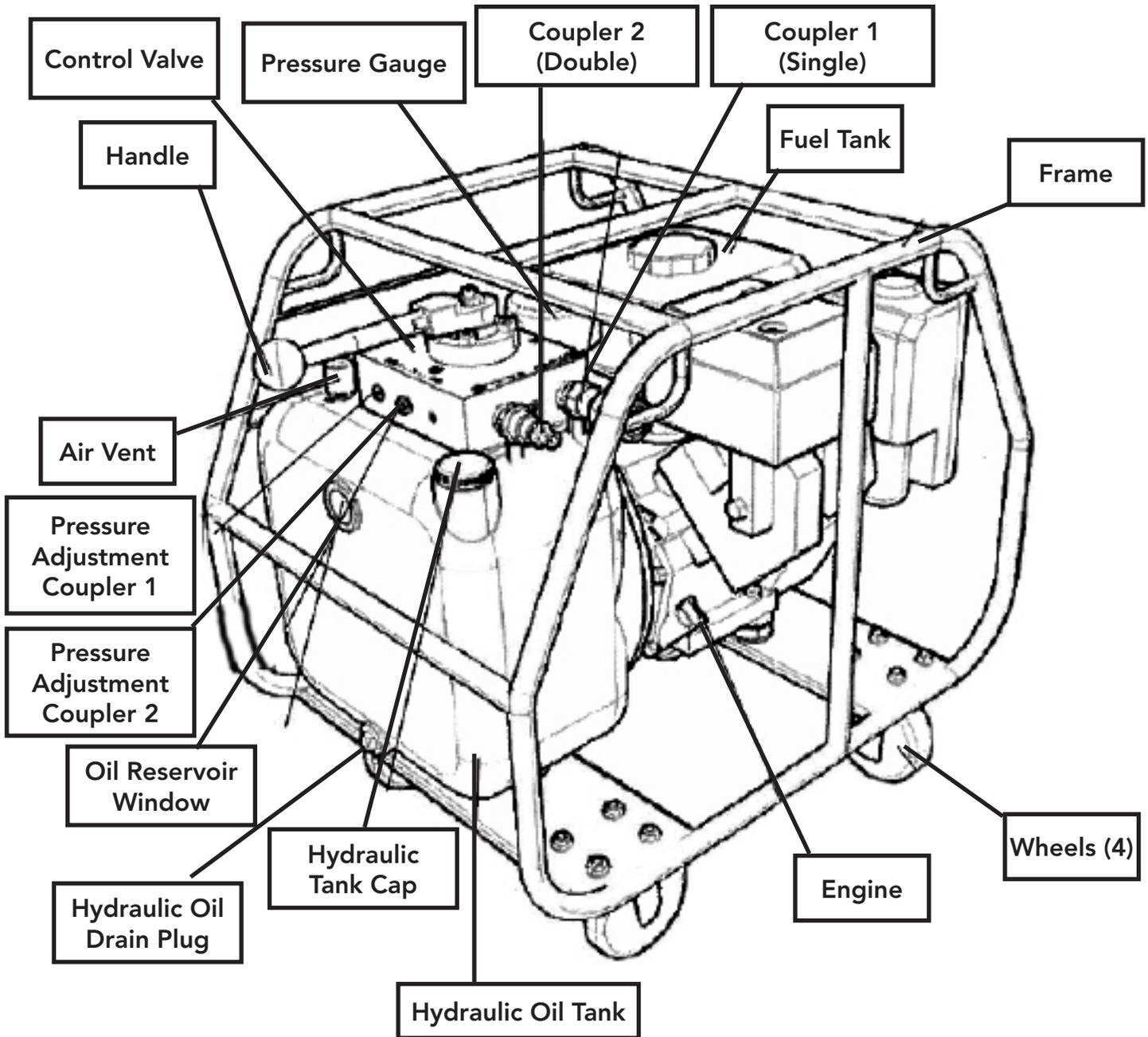
1. The HPM-P3 pump can be used as a Single-Acting or Double-Acting Pump. You can operate 1 or 2 Single-Acting heads or 1 Double-Acting head.
